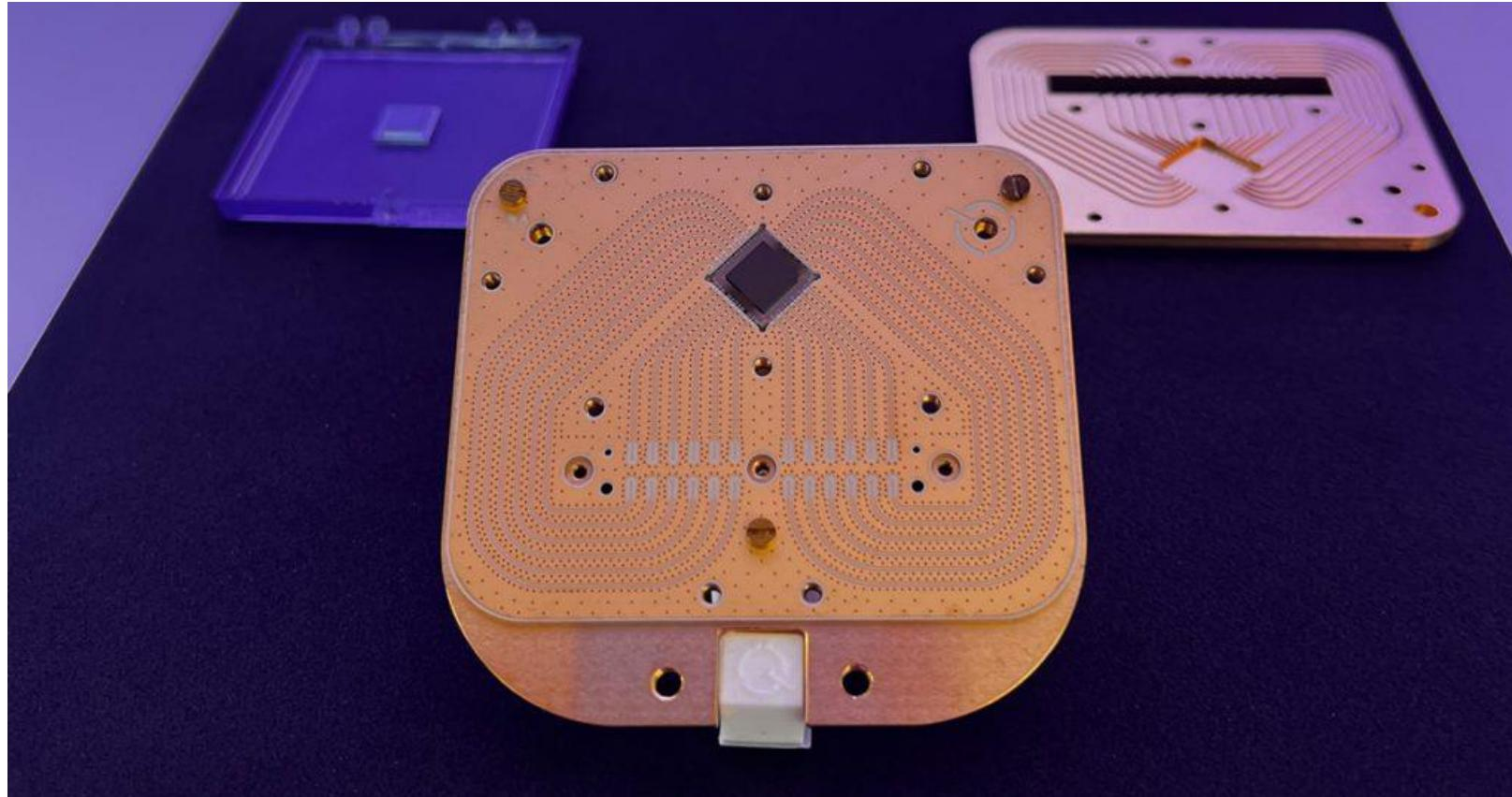
*The new VLQ quantum computer contains 24 superconducting qubits in a star-shaped topology and will be available to users in Denmark!*
